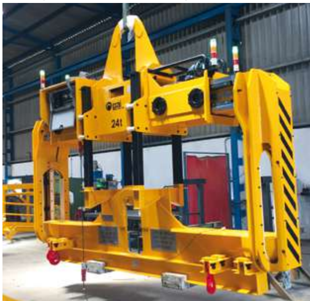
Special grab load attached to spreader beam Pinza especial unida a balancín de carga
