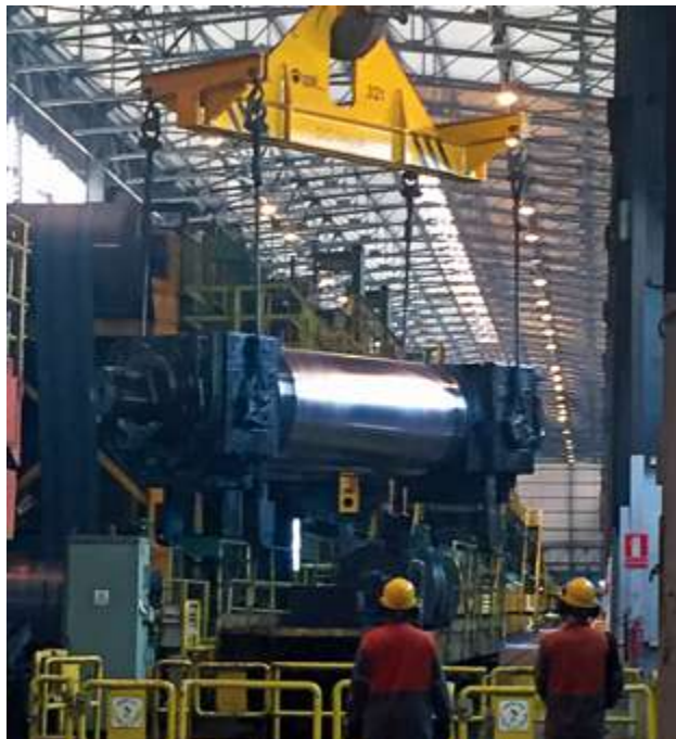
Spreader with motorized rotation, 60 tonnes Balancín con giro motorizado, 60 tn
