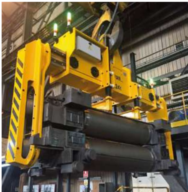
Special grab load attached to spreader beam Pinza especial unida a balancín de carga
